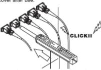
3.Push the Outer Shell to start cleaning the SC connector end face.A "click" sound indicates end of cleaning process. Close the cover after use.
