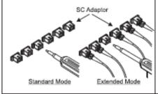
2.Insert SC connector into the Guide Cap
